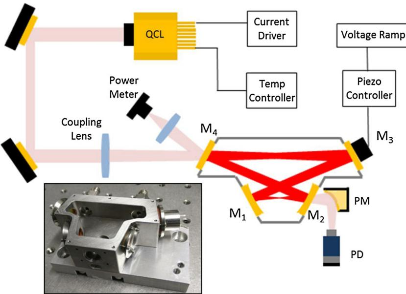
**Fig. 2.** Schematic of the experimental setup employed for coupling a collimated laser beam into the bow-tie cavity. Inset: a picture of the stainless-steel housing containing the four mirrors forming the bow-tie cavity. QCL – Quantum cascade laser. PM – Parabolic Mirror. PD – Pyroelectric Detector.
