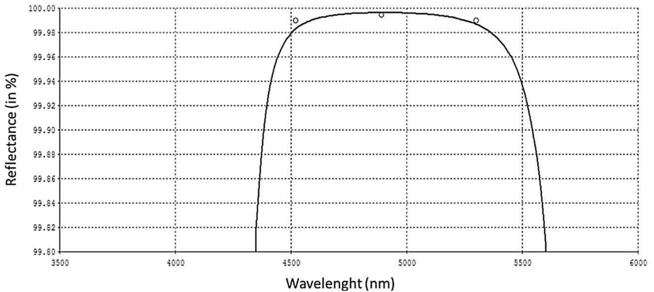
**Fig. 3.** Mirror reflectance spectrum provided by Lohstar, Optics Inc. in the range between 3.5  $\mu\text{m}$  and 6.0  $\mu\text{m}$ . The three dots are located at 4520 nm, 4890 nm and 5300 nm corresponding to a reflectivity of 99.99%, 99.995% and 99.99%, respectively.
