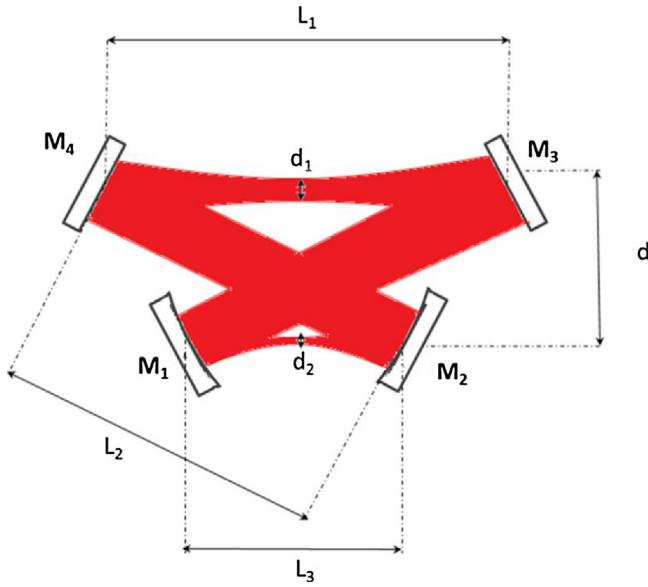
**Fig. 1.** The bow-tie resonator geometry employed in the reported study. The plane mirrors are separated by a distance  $L_1$ . The distances between  $M_1$  and  $M_3$  and  $M_2$  and  $M_4$  are identical and denoted as  $L_2$ . The spacing between the two concave mirrors  $M_1$  and  $M_2$  is denoted as  $L_3$ . The width of the cavity is denoted as  $d$ .
