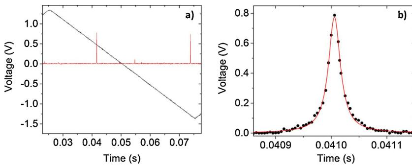
**Fig. 4.** (a) The cavity transmission signal obtained at atmospheric pressure (red solid line) when a voltage ramp (black solid line) is applied to the piezo controller in order to cover one free spectral range of the cavity; (b) Enlarged view of one of the transmission peaks of the cavity (black dots) and related Lorentzian best fit (red solid line). (For interpretation of the references to colour in this figure legend, the reader is referred to the web version of this article.)
