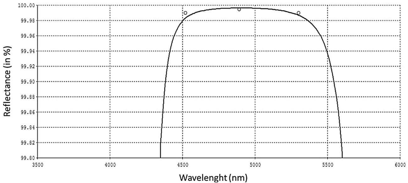
**Fig. 3.** Mirror reflectance spectrum provided by Lohnstar, Optics Inc. in the range between 3.5  $\mu\text{m}$  and 6.0  $\mu\text{m}$ . The three dots are located at 4520 nm, 4890 nm and 5300 nm corresponding to a reflectivity of 99.99%, 99.995% and 99.99%, respectively.
