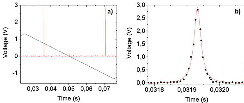
**Fig. 5.** (a) Transmission of the bow-tie optical cavity containing air sample at 90 Torr (red solid line) and the voltage ramp (black solid line) applied to the piezo controller; (b) Enlarged view of one of the cavity transmission peaks (black dots) and the related Lorentzian fit (red solid line). (For interpretation of the references to colour in this figure legend, the reader is referred to the web version of this article.)
