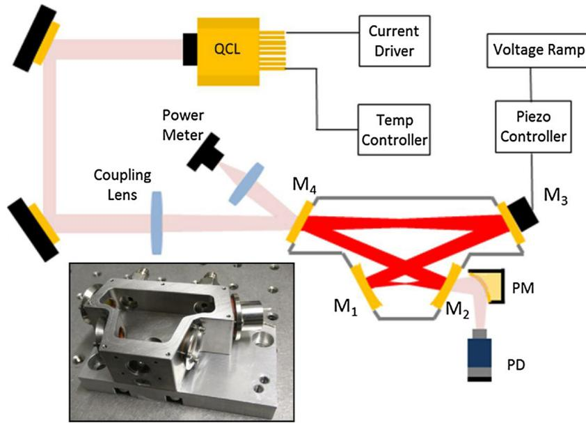
**Fig. 2.** Schematic of the experimental setup employed for coupling a collimated laser beam into the bow-tie cavity. Inset: a picture of the stainless-steel housing containing the four mirrors forming the bow-tie cavity. QCL – Quantum cascade laser. PM – Parabolic Mirror. PD – Pyroelectric Detector.
