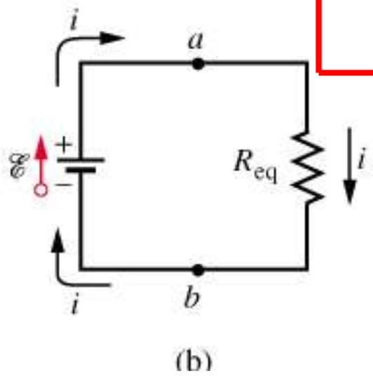
$$R_{eq} = \left( \frac{1}{R_1} + \frac{1}{R_2} + \frac{1}{R_3} \right)^{-1}$$
