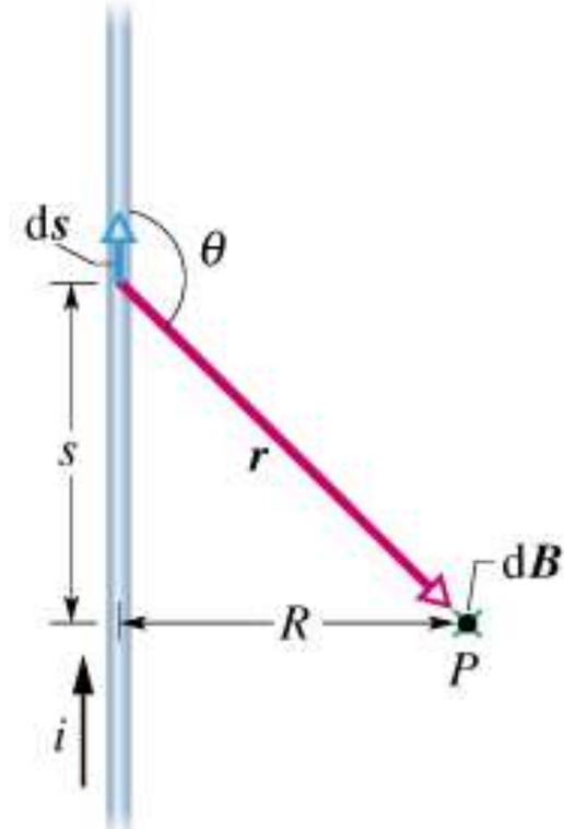
$$|\vec{B}| = \int_0^\pi \left( \frac{\mu_0}{4\pi} \right) \frac{i \cdot \sin \vartheta}{R} d\vartheta = \left( \frac{\mu_0}{4\pi} \right) \frac{i}{R} \int_0^\pi \sin \vartheta \cdot d\vartheta =$$
