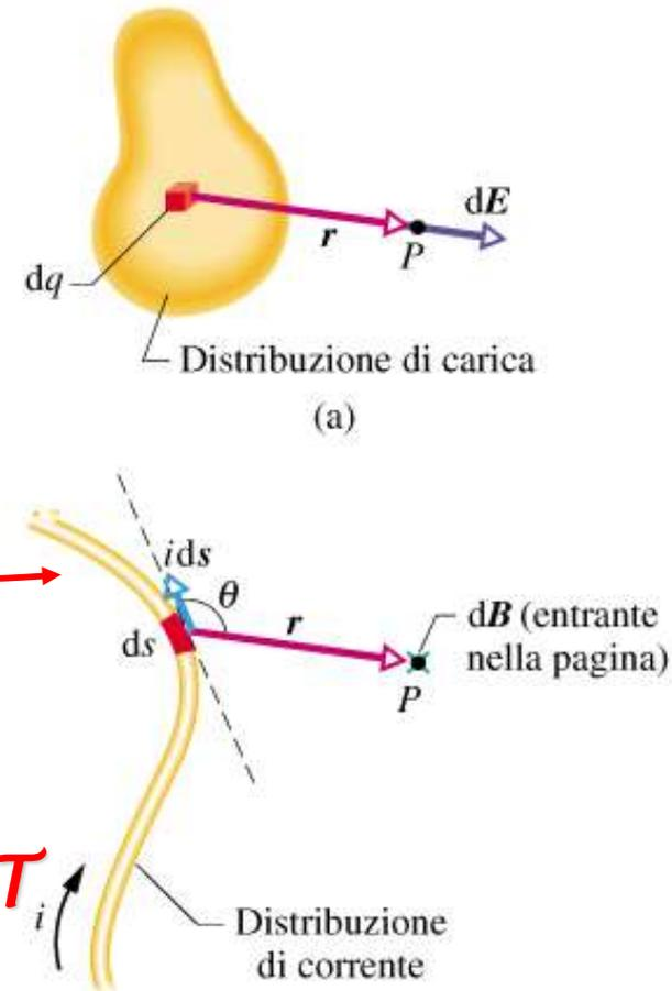
$$d\vec{B} = \frac{\mu_0}{4\pi} \frac{i d\vec{s} \times \hat{u}_r}{r^2} \longrightarrow \left\{ \begin{array}{l} j = \frac{i}{\Sigma} \\ \vec{j} = (nq\vec{v}_d) \end{array} \right.$$
