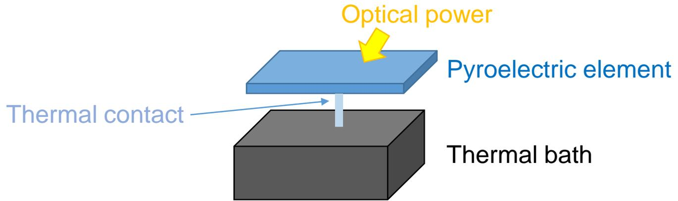
The pyroelectric material is connected by a weak thermal contact with thermal conductance  $G$  [W/K] to a thermal bath (*heat sink*) at temperature  $T_0$ . Suppose there are no leak channels for heat dissipation.
