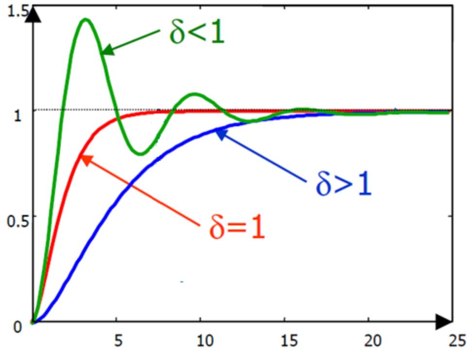
With  $\delta \geq 1$ , the sensor response is comparable to that of a first order system.
