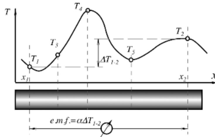
A temperature gradient between any arbitrary points defines an electromotive force ( $emf$ ) between these points.
