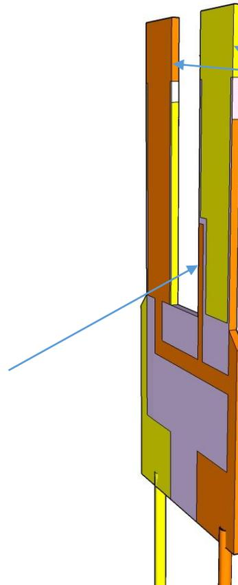
*Wrap around at the top of the prong to connect the two opposite front surfaces*
