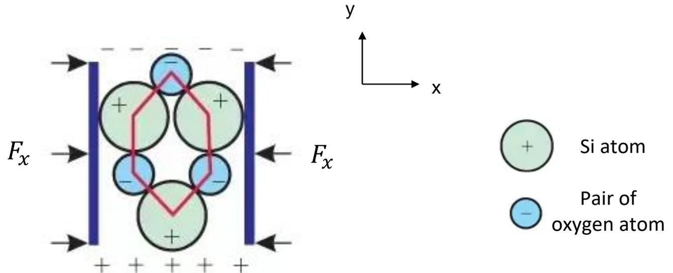
This simple model illustrates that crystalline material can develop electric charge on its surface in response to a mechanical deformation. .
