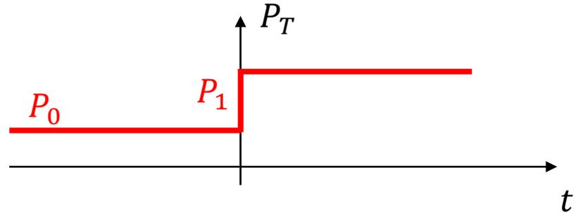
$P_0$  is the power incident on the sensing element (external light), not due to the amount to be measured,  $P_1$ .
