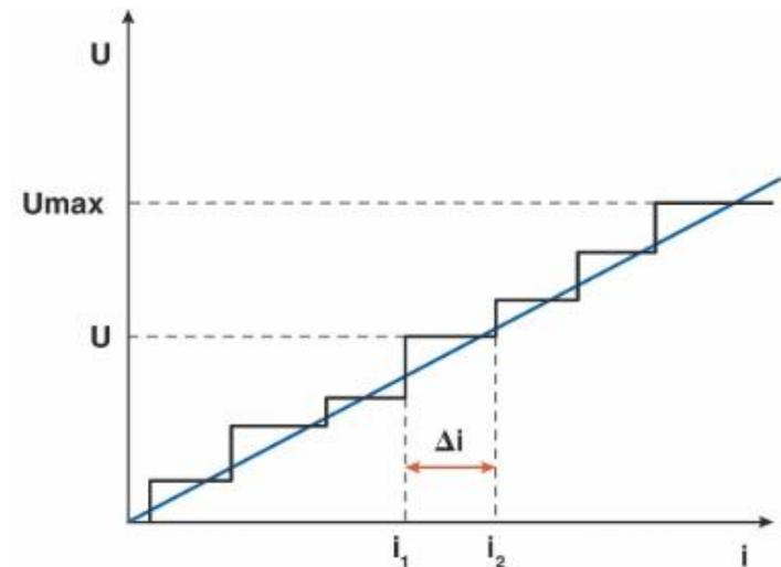
For instance, for the angular sensor having  $270^\circ$  FS, the  $0.5^\circ$  resolution may be specified as 0.181% of FS. It should be noted that the step size may vary over the range, hence, the resolution may be specified as typical, average, or “worst.”
