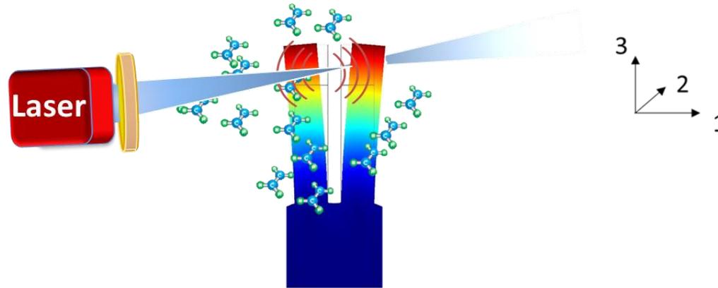
The situation can be schematized assuming that a mechanical stress  $\vec{T}$  is applied on one prong along the direction 1, while a mechanical stress  $-\vec{T}$  is applied on the same direction on the other prong. This will generate a charge along the direction 1 and a charge in the direction 2, as schematized here:
