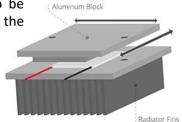
A complete thermoelectric cooling system includes the Peltier element, the heat sink, temperature sensors to monitor hot and cold plates, and a control unit to ensure that the correct current is supplied to maintain the desired temperature difference through the module.
