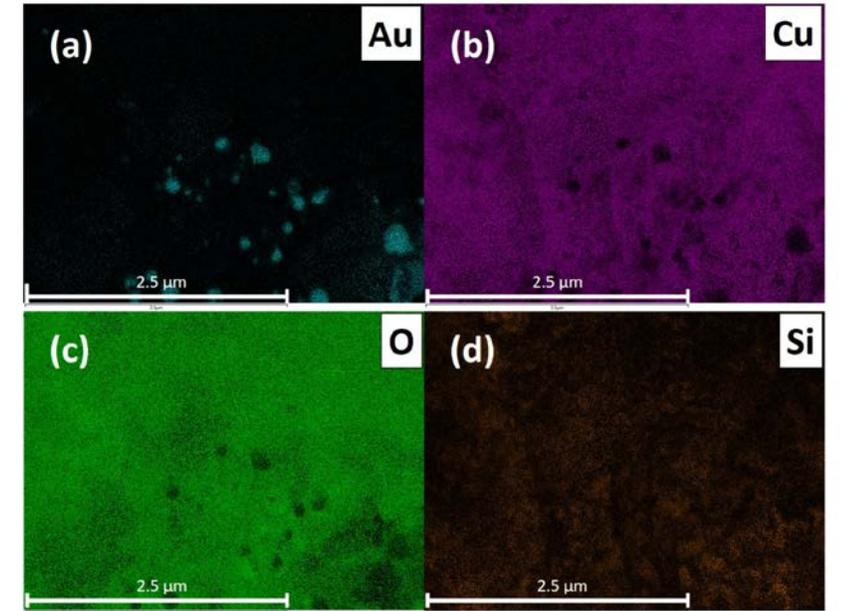
Figure 4. Elemental mapping of a 4 μm × 4 μm section on the copper oxide surface with 5 keV (primary beam energy). (a) Au elemental map, (b) Cu elemental map, (c) O elemental map and (d) Si elemental map.
