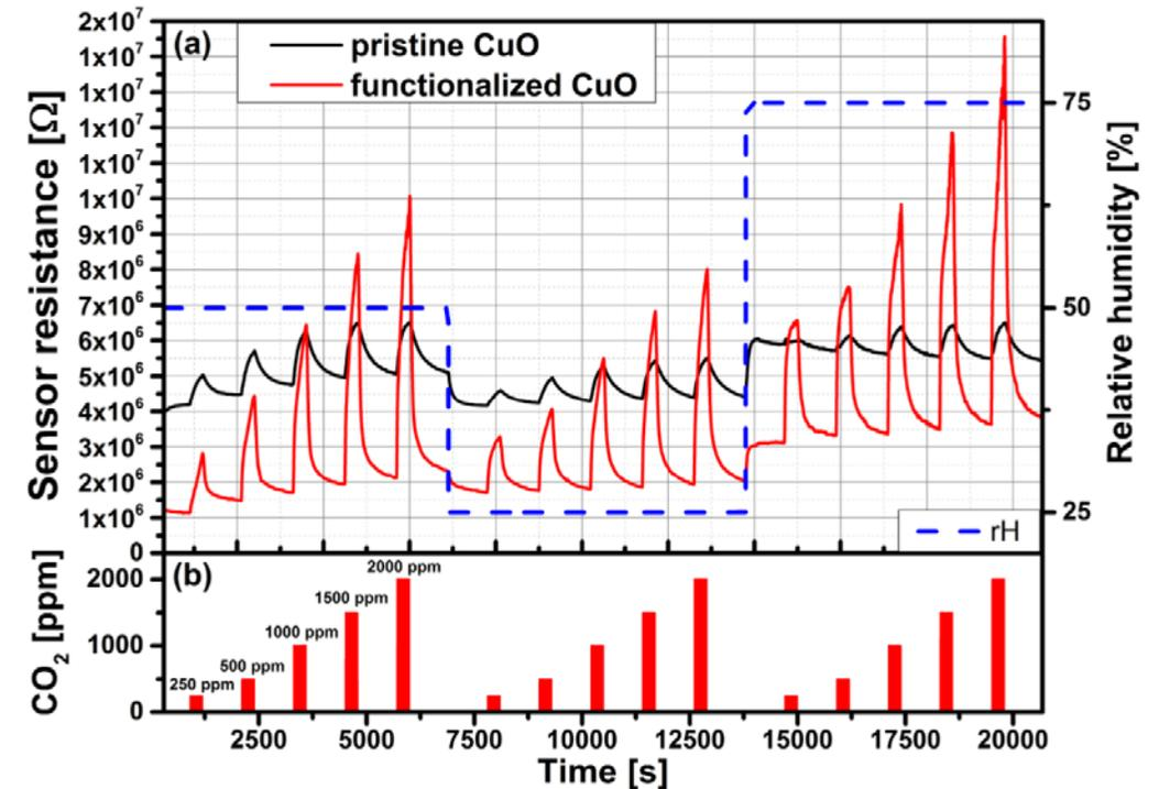
Figure 6. (a) Carbon dioxide measurement of the pristine and functionalized CuO gas sensors at an operation temperature of 300 °C and rH levels of 25%, 50% and 75%. (b) CO<sub>2</sub> gas pulses: 250 ppm, 500 ppm, 1000 ppm, 1500 ppm and 2000 ppm.
