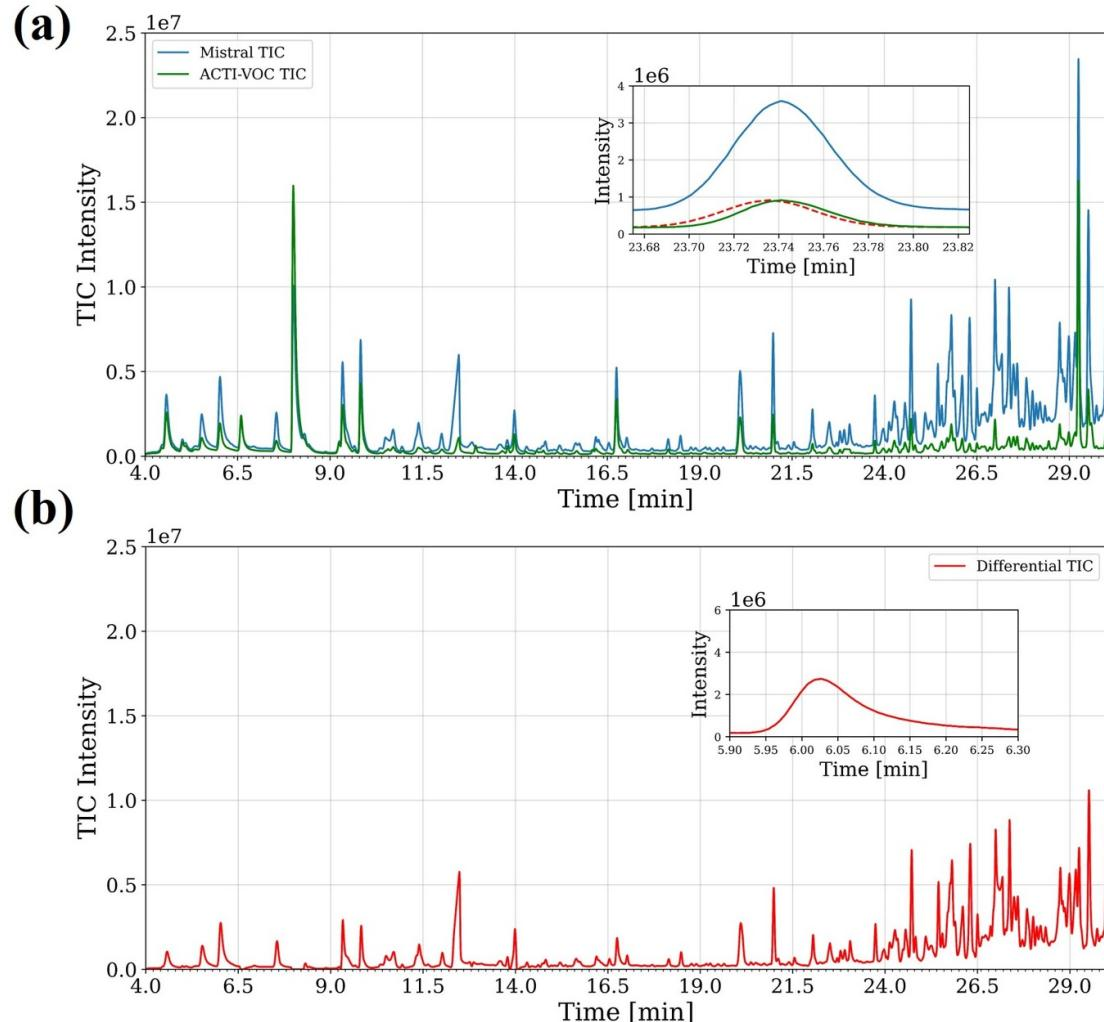
**Figure 2.** (a) Total ion chromatograms (TIC) obtained using the Mistral sampler (blue solid line) and the ACTI-VOC pump (green solid line) after alignment processing. In the inset, in red is shown the ACTI-VOC pump TIC prior to the alignment (red dashed line) (b) Differential TIC (red solid line).
