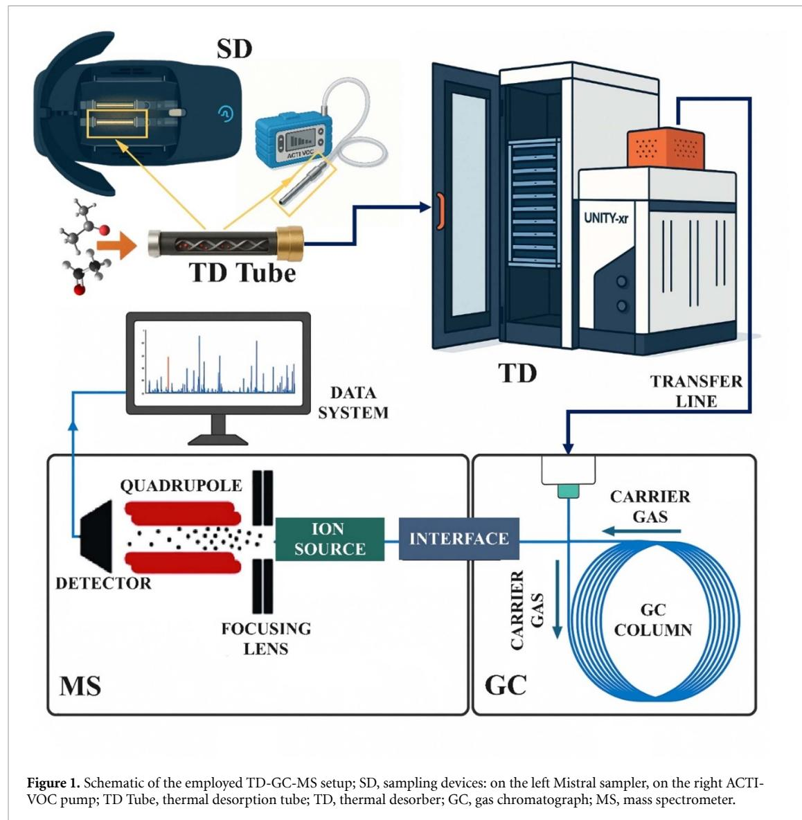
**Figure 1.** Schematic of the employed TD-GC-MS setup; SD, sampling devices: on the left Mistral sampler, on the right ACTI-VOC pump; TD Tube, thermal desorption tube; TD, thermal desorber; GC, gas chromatograph; MS, mass spectrometer.
