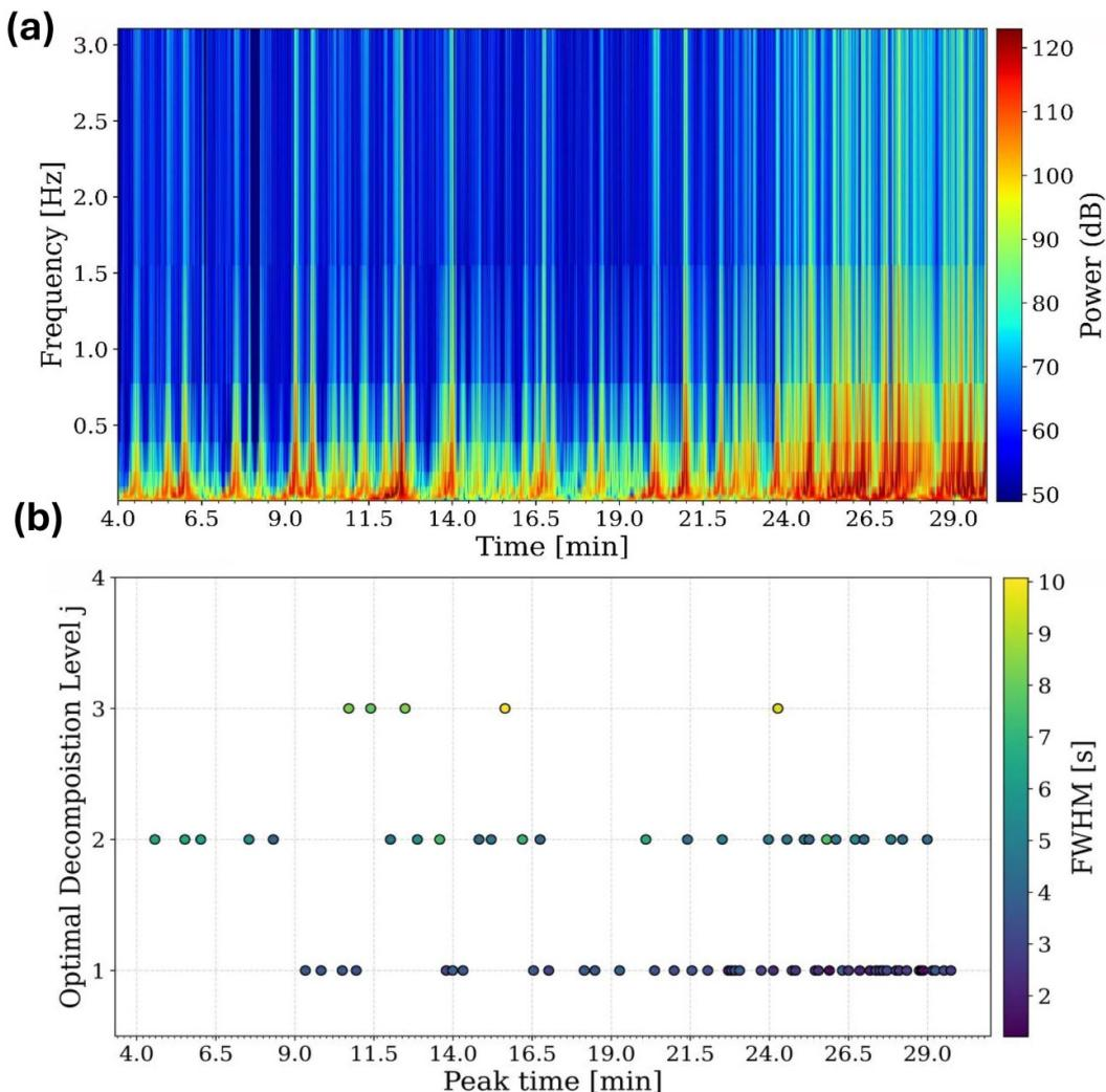
**Figure 3.** (a) Multiscale scalogram of the stationary wavelet transform (levels 1–11) using a Daubechies-3 wavelet. (b) Optimal decomposition level compared to the peaks FWHM.
