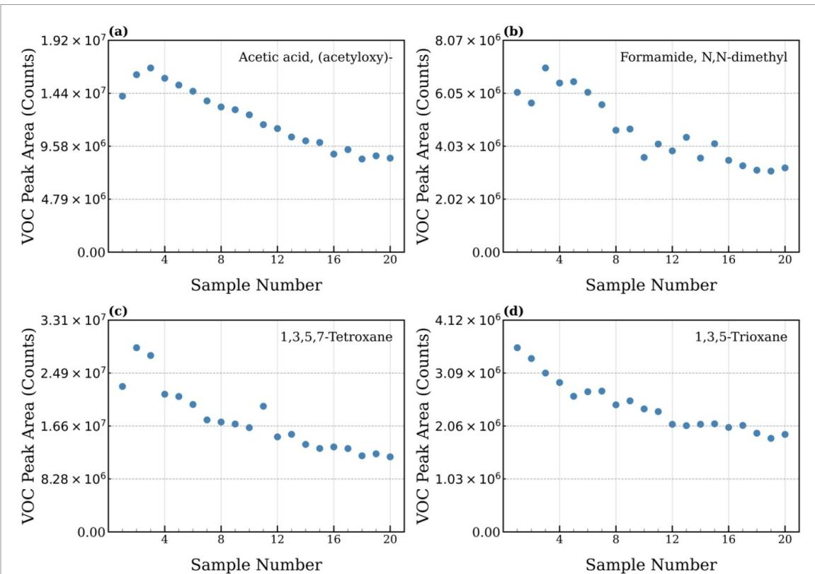
**Figure 7.** Time-resolved emission profiles for the four artificial VOCs across 20 Mistral replicates in Session 2. Compounds: (a) 1,3,5,7-Tetroxane, (b) 1,3,5-Trioxane, (c) (Acetyloxy)acetic acid, and (d) N,N-Dimethylformamide.
