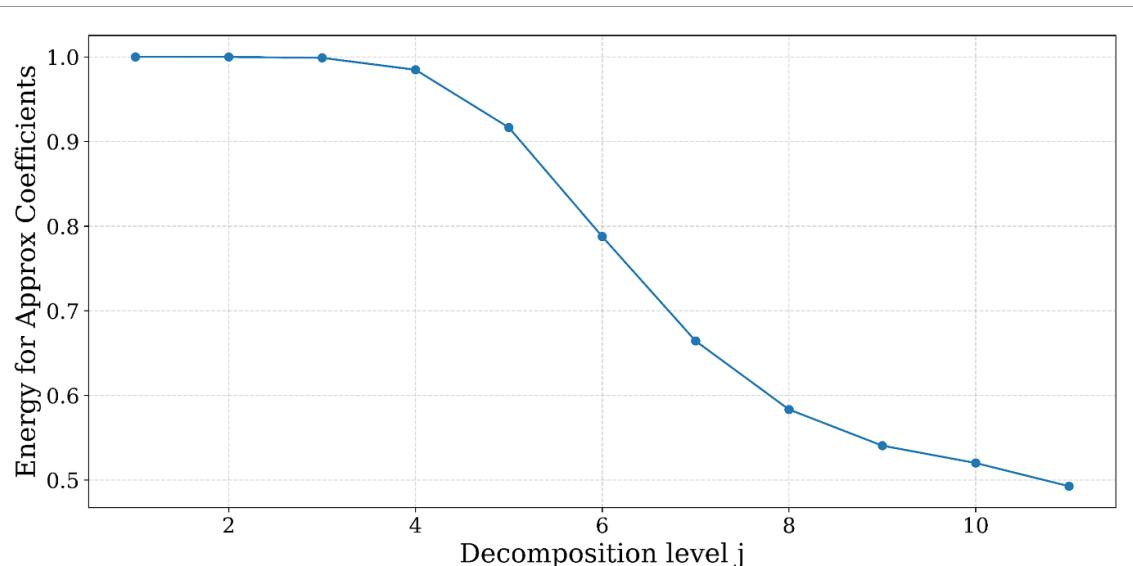
Figure 4. Energy of approximation coefficients as a function of the wavelet decomposition level ( $j$ ).
