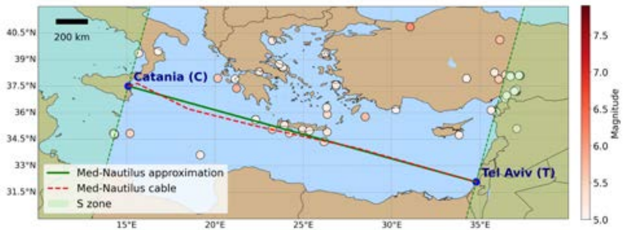
Figure 5. The Med-Nautilus section of interest. Med-Nautilus comprises 5,729 km of cable, with a design capacity of 3.84 Tb/s distributed across six fiber optic pairs. In this work, we focused on the Catania (ITA) - Tel Aviv (ISR) section. This cable section is represented by the dashed red line: the actual position of the cable may slightly differ from this representation, since cable precise coordinates are not publicly available due to security reasons. The cable section was approximated by the geodesic CT (green continuous line); this section has length above 2,500 km. The circles shown in the figure represent the 60 seismic events with magnitude M \geq 5 that occurred in the Mediterranean area between June 1 st , 2022 and November 30 th , 2024. The aim of this research work is studying the changes in the State of Polarization (SOP) of the electromagnetic signal in the Med-Nautilus CT fiber cable section due to the mechanical stress derived from P- and S- seismic waves. The two geodesics passing through C and T (green dashed lines) create a sort of wedge-shaped region which is our zone of interest; the outer region is denoted as S zone.
